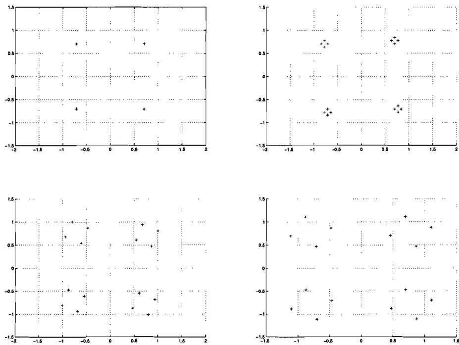
Figure 4.4: Effect of IQ imbalance in transmitter and receiver on observed QPSK constellation; upper left: no IQ imbalance; upper right: TX imbalance 10%, 5°, lower left: RX imbalance 10%, 5°, lower right: both TX and RX imbalance 10%, 5°
