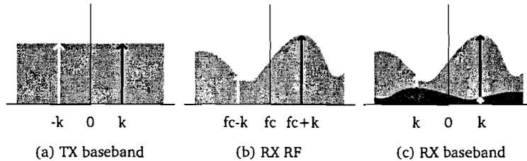
Figure 4.2: Influence of receiver caused IQ imbalance on received OFDM signal spectrum
