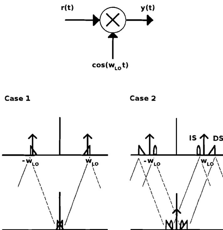
Figure 3.1: Mixing a real signal with a cosine. In case 1, the frequency  $\omega_{LO}$  is equal to the center frequency of the desired signal, and in case 2,  $\omega_{LO}$  is not equal to the center frequency of the desired signal.
