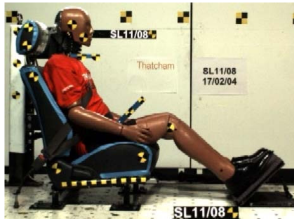
Figure 3 – Test setup with BioRID on seat E
