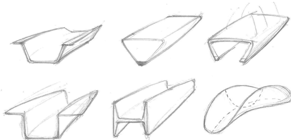
Fig. 8: Variable bridge cross-sections
