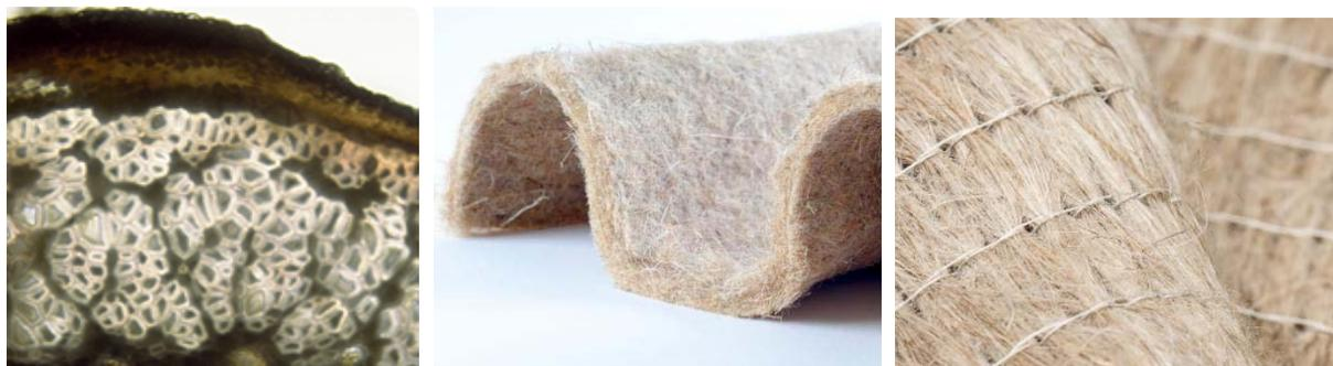
Fig. 1: Cross-section of hemp fibres under the microscope
