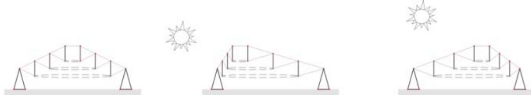
Fig. 17. Concept of sliding dome for low and high sun top view of kinetic tensegrity dome
