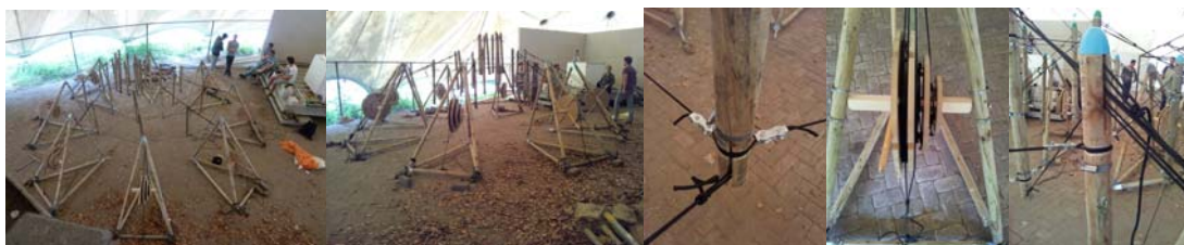
Fig. 27. (a + b) movement of the dome, (c + d + e) details of the dome and the hand-powered pulleys.
