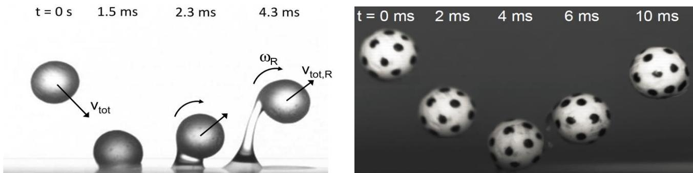
Figure 1: Comparison of collision dynamics of glass particles (left) and aluminum oxide particles (right) impacting on a glass plate covered by a liquid layer of 400  $\mu\text{m}$  and 100  $\mu\text{m}$  layer thickness, respectively.
