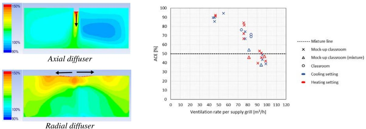
Figure 1: Local air change index in a living room with the same air flow rate but different diffusers (higher value is better; ±100% is mixing) [left]; air change efficiency (ACE) as function of the air supply rate [right].
