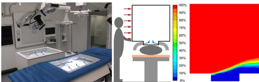
Figure 2: Local ventilation solution at wound area and instrument table [left]; CFD assessment of the relative particle concentration (0% is optimal) [right].
