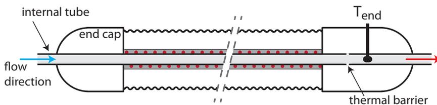
Figure 6.5: Heating tube schematic
