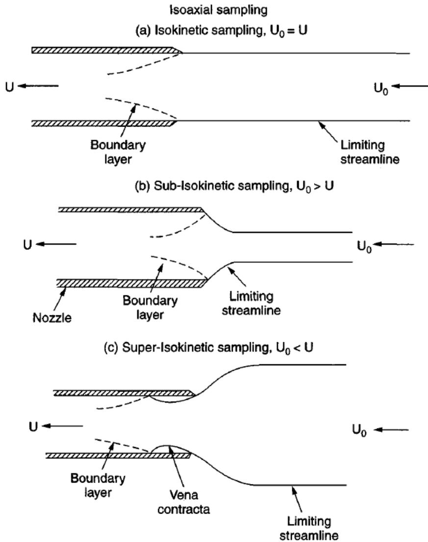
Figure 5.1: Schematic of isoaxial sampling with thin walled nozzle. The flow characteristics for (a) iso-, (b) sub and (c) super-kinetic sampling conditions are displayed. obtained from *Aerosol Measurement: principles, techniques and applications*, 2nd edition, A Baron and K. Willeke, Wiley Interscience, 2001
