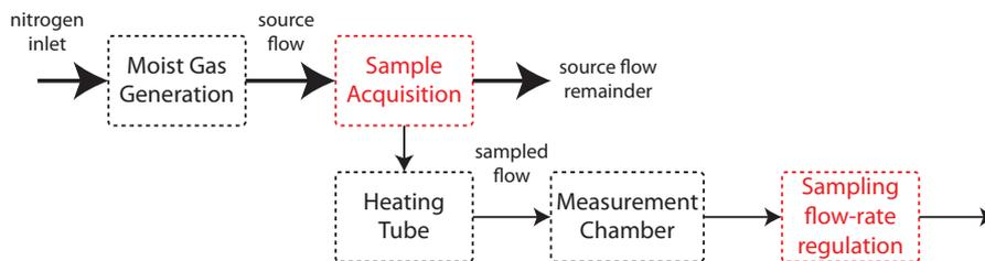
Figure 6.7: Schematic flow chart of the entire continuous measurement setup.
