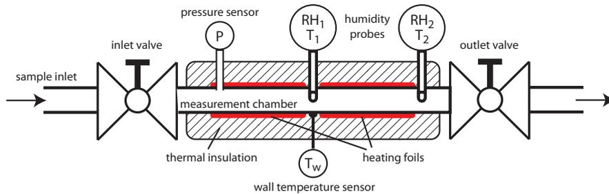
Figure 6.1: Heating tube schematic
