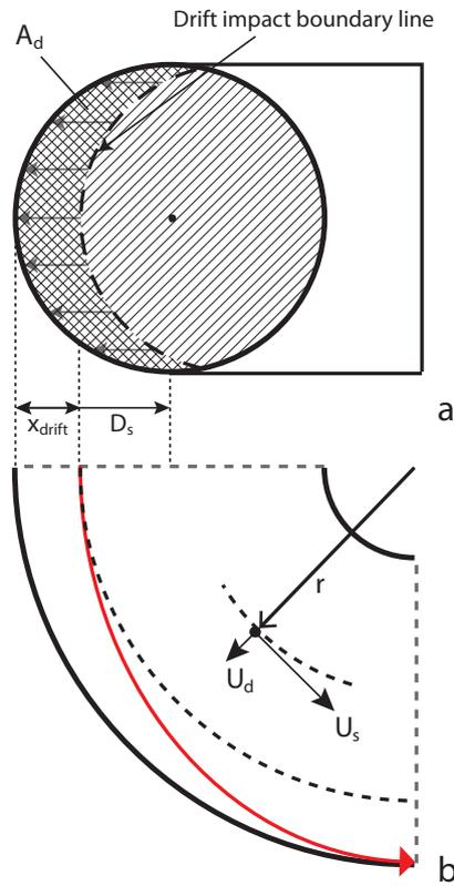
Figure 5.3: Inertial deposition in a quarter bend.
