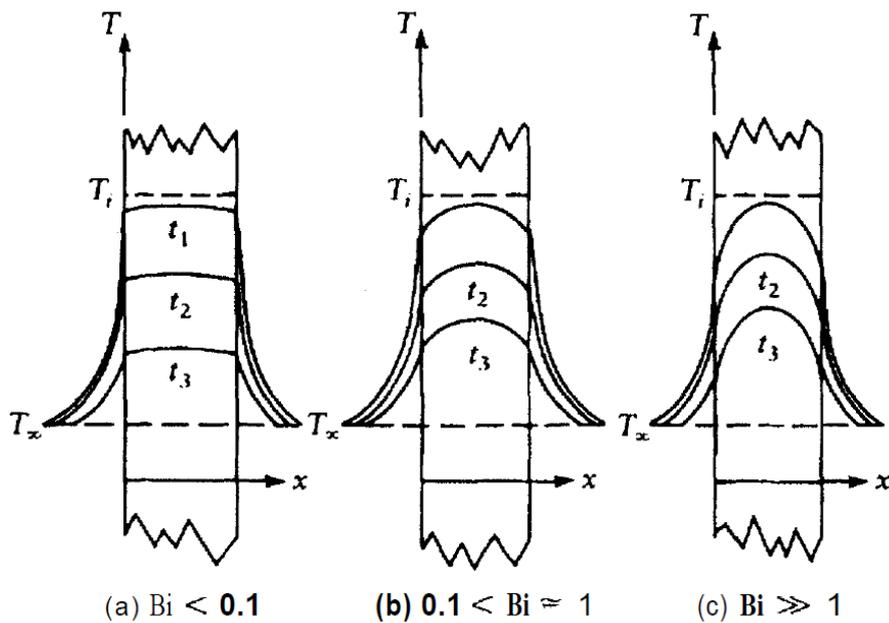
Figure 4.1: Temperature gradients of cylindrical volumes at extreme values (a) and (c), and an intermediate situation (b).  $T_i$  is the initial temperature profile and the development at three later moments in time  $t_1, t_2$  and  $t_3$  are shown for the three situations. (taken from Janna 2000 [11], pg192)
