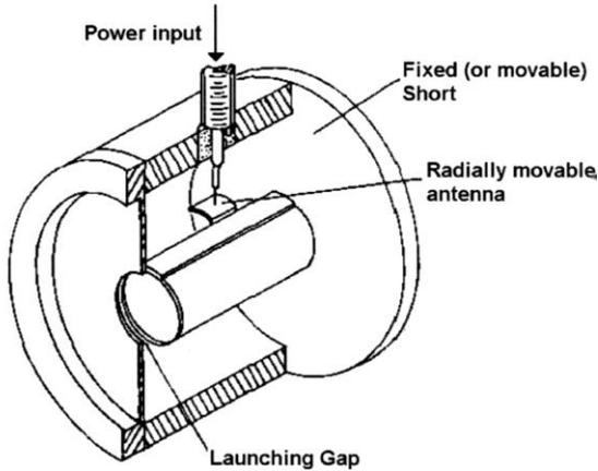
Figure 1: A cross-section of the surfatron. Components have been named. [2]
