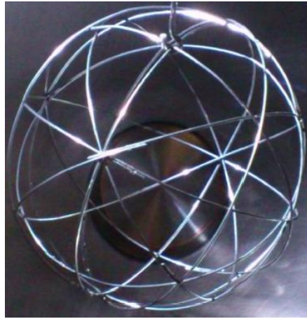
Figure 7.3: The regular grid. 9 circular wires welded together to form a spherical grid.
