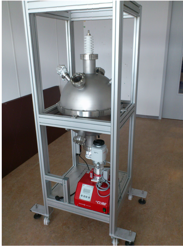
Figure 7.2: A picture of the vacuum vessel with the grid inside. The pump also can be seen at the bottom of the picture.
