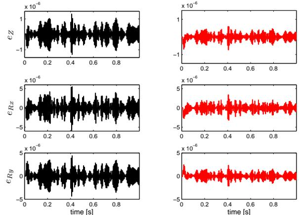
**Figure 2:** Measured time domain responses: controller based on classical weighting functions  $C^{\text{class}}$  (black) and  $C^{\text{mimo}}$  (red) based on the proposed multivariable weighting.
