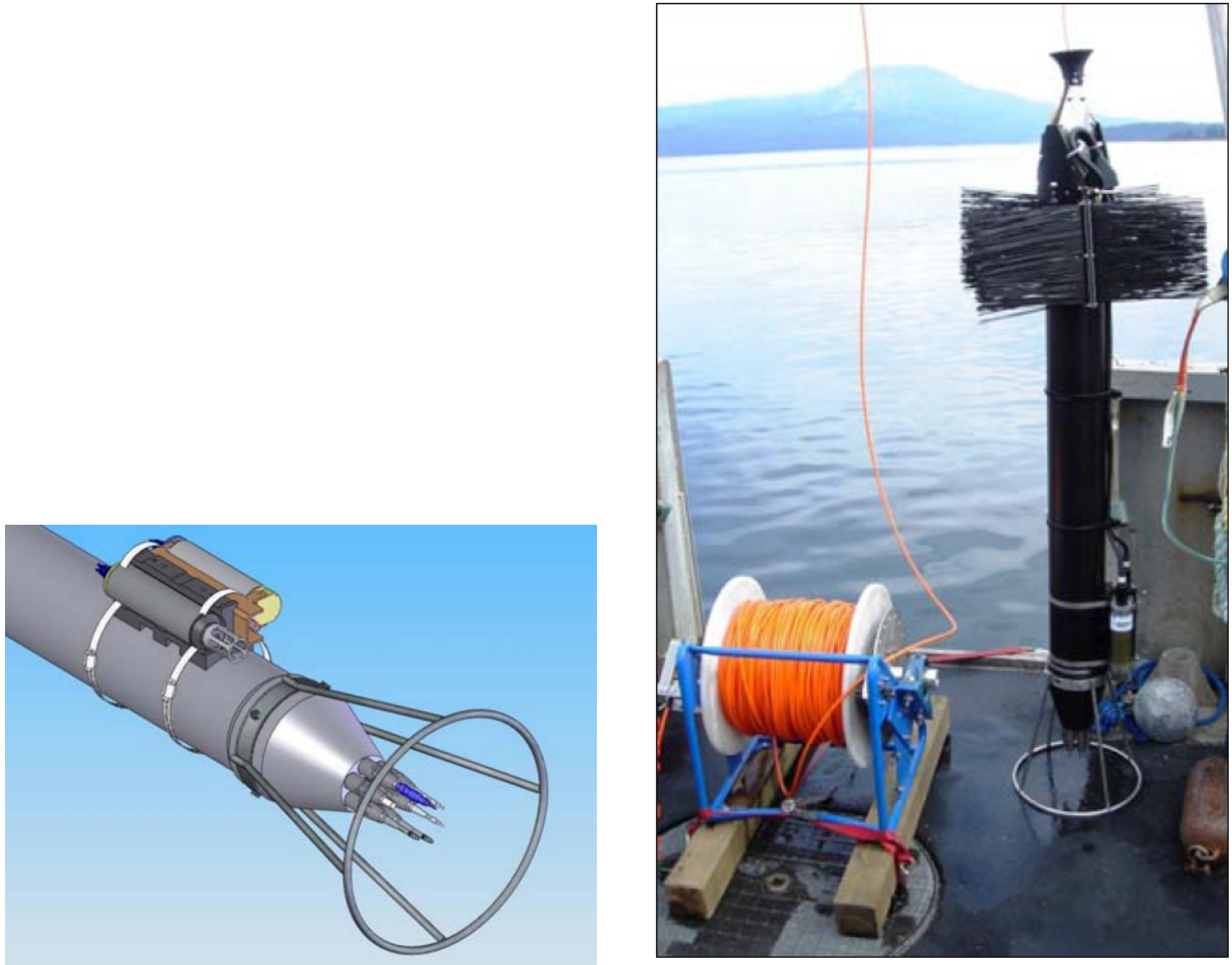
Figure 3.1: The VMP-500 profiler with its sensors and a cage protecting the sensors once the profiler hits the sea floor.
