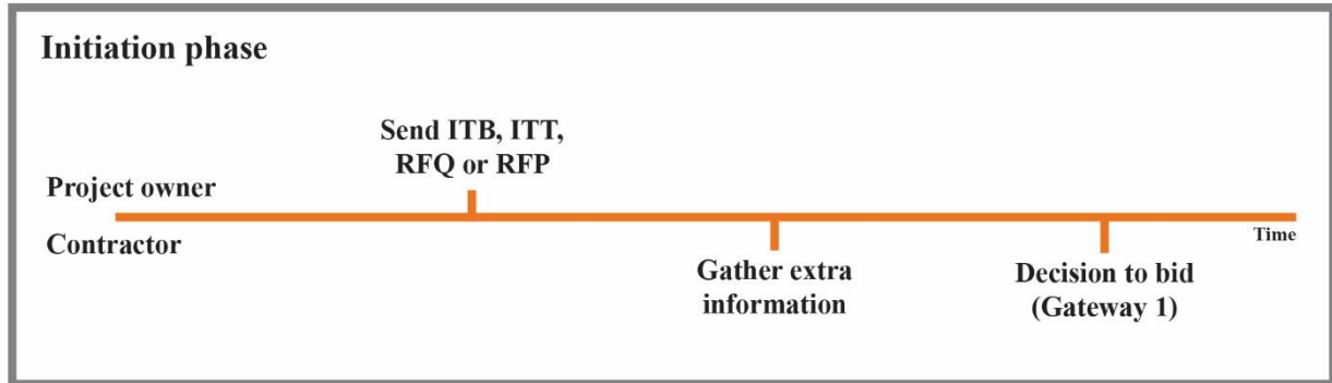
Figure A3. Illustration of the initiation phase, including contractor activities below the timeline, and project owner activities above the timeline. (ITB = Invitation to Bid, ITT = Invitation to Tender, RFQ = Request for Quotation, and RFP = Request for Proposal)
