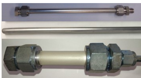
Fig. 1. Membranes from top to bottom, 7 Nm sealed swagelok, finger like and 14 Nm sealed swagelok membrane.
