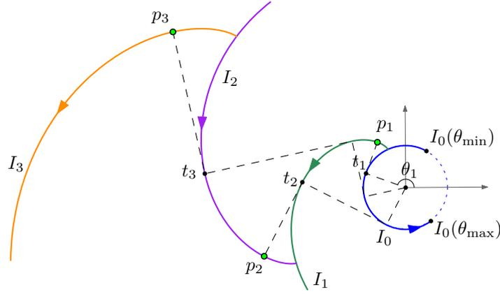
■ **Figure 2** Circular arc  $I_0(\theta)$ , and three involutes  $I_1(\theta)$ ,  $I_2(\theta)$ , and  $I_3(\theta)$ : for each  $i$ ,  $I_i(\theta)$  is an involute about  $I_{i-1}(\theta)$  that passes through point  $p_i$ . The arrows designate the direction of growth of the parameter  $\theta$  (they are not necessarily consistent with the direction of a self-approaching path).
