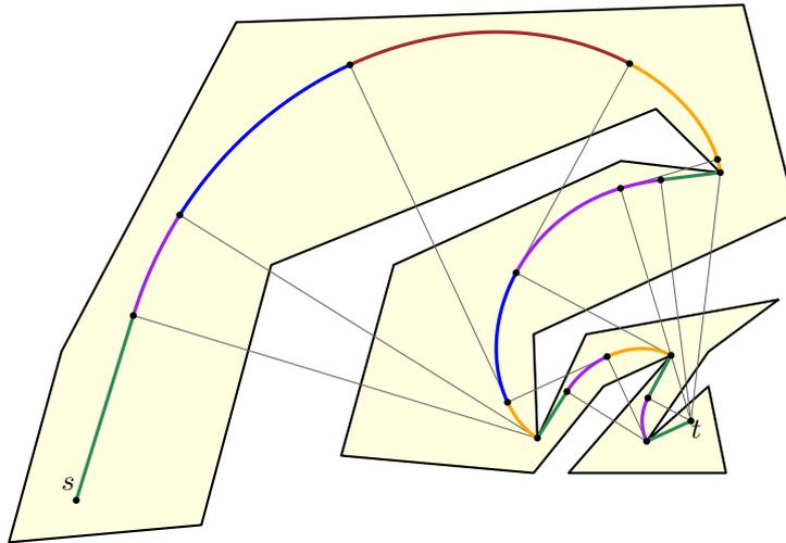
■ **Figure 5** Shortest self-approaching path from  $s$  to  $t$  consists of straight-line segments, circular arcs, and involutes of a circle of some order. Straight segments are shown in green, circular arcs in purple, involutes of a circle of first order in orange, involutes of a circle of a second order in blue, and involutes of a circle of third order in brown.
