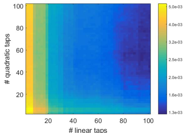
**Fig. 4:** Full two-dimensional tap-sweep for a blind feedforward equalizer with added quadratic taps<sup>2</sup> working on the received signal after 93 km of transmission with 23 dB OSNR. An equalizer with 21 linear taps and 11 quadratic taps was used in the transmission experiments.
