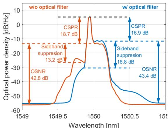
**Fig. 3:** Optical spectrum (back-to-back), with and without the optical tunable filter, showing carrier-to-signal power ratio (CSPR), sideband suppression and optical signal-to-noise ratio (OSNR). Measured with 0.05nm resolution.
