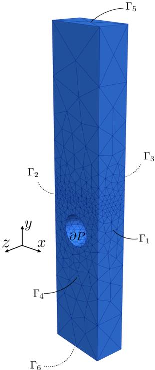
Fig. 1: An example of the computational mesh indicating the boundaries (note: in the actual computations the mesh is much more refined).
