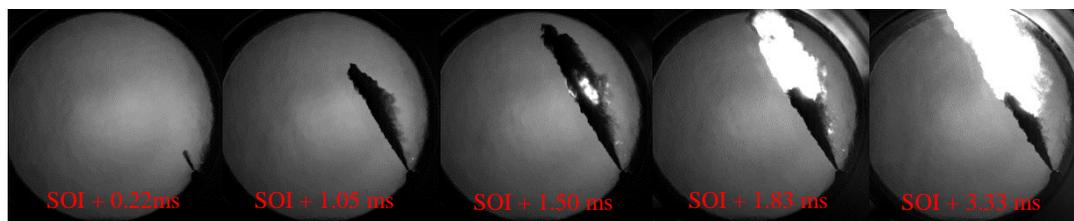
Figure 5. Injection and combustion progress in shadowgraphy images, with the 1<sup>st</sup>, 2<sup>nd</sup> and 3<sup>rd</sup> shots taken shortly after the start of injection, auto-ignition and establishment of quasi-steady flame, respectively
