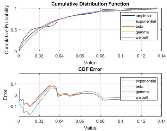
Figure D.2: Top 5 Cumulative distribution function fits for  $C_1$  based on AICc
