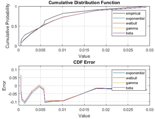
Figure D.12: Top 5 Cumulative distribution function fits for  $C_6$  based on AICc
