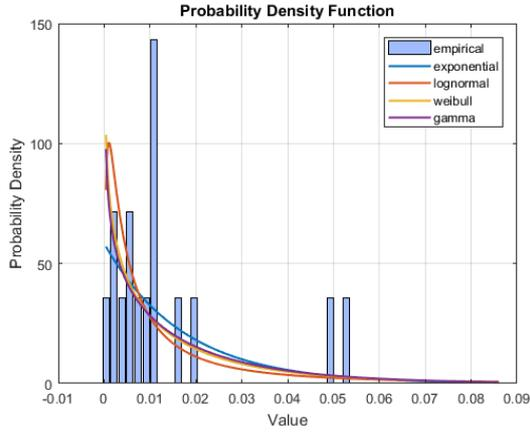
Figure D.9: Top 5 Probability density function fits for  $C_5$  based on AICc
