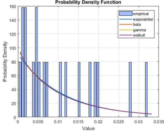
Figure D.3: Top 5 Probability density function fits for  $C_2$  based on AICc
