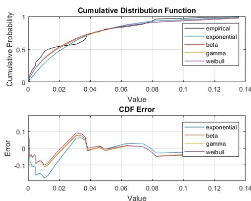
Figure 4.3: Top 5 Cumulative distribution function fits for  $F_1$  based on AICc
