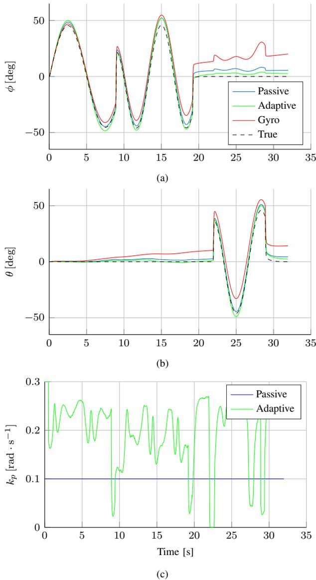
Fig. 4. Simulation results for  $k_0 = 0.3 [\text{rad} \cdot \text{s}^{-1}]$ ,  $\xi = 0.4 [-]$ ,  $h = 0.5 [\text{s}]$ ,  $k_p = 0.1 [\text{rad} \cdot \text{s}^{-1}]$ . The top and middle plot show the angular estimates resulting from the non-adaptive (blue) and adaptive filter (green), gyroscope integration (red) and the actual angle (dashed black) for the pitch and roll angles, respectively. The bottom plot shows the adaptive (green) and fixed gain (blue) over time.
