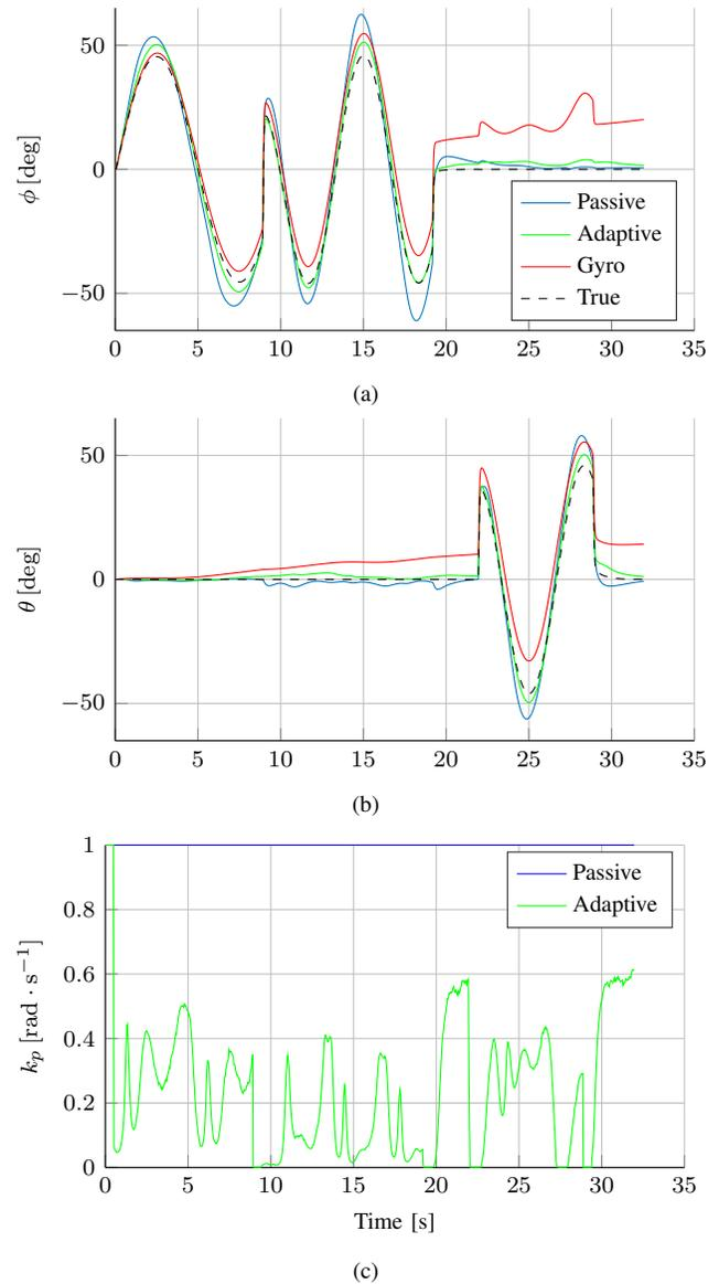
Fig. 5. Simulation results for  $k_0 = 1 [\text{rad} \cdot \text{s}^{-1}]$ ,  $\xi = 2 [-]$ ,  $h = 0.5 [\text{s}]$ ,  $k_p = 1 [\text{rad} \cdot \text{s}^{-1}]$ . The top and middle plot show the angular estimates resulting from the non-adaptive (blue) and adaptive filter (green), gyroscope integration (red) and the actual angle (dashed black) for the pitch and roll angles, respectively. The bottom plot shows the adaptive (green) and fixed gain (blue) over time.
