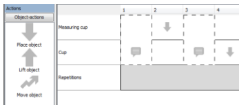
Figure 3: Close-up of the timeline based visual programming interface for therapy exercises.
