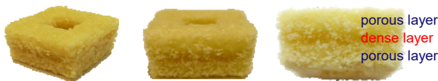
Figure 2: A multi-texture 3D printed food product from specifically designed cake mix created with powderbed printing and a post-processing baking step.
