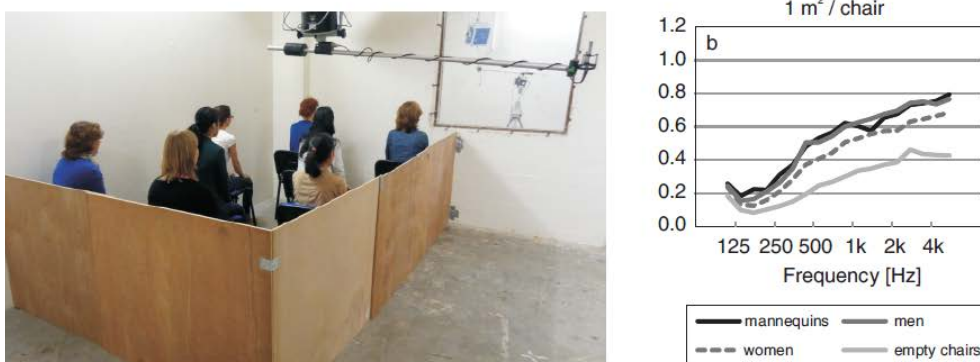
Fig 2. Results of sound absorption measurements in the reverberation room.
