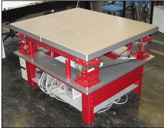
Figure 8: Benchmark active vibration isolation system (AVIS).
