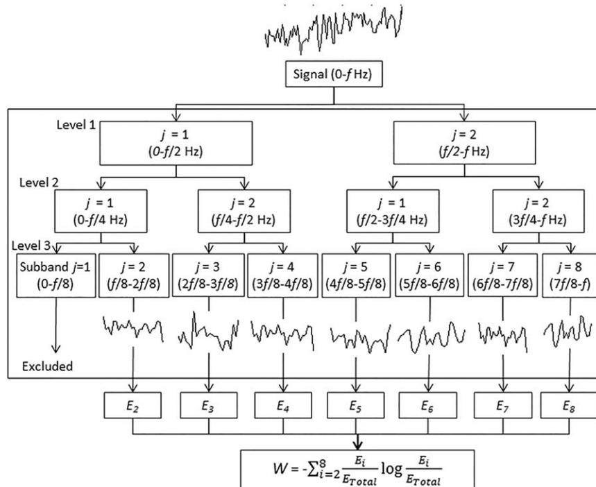
**FIGURE 1:** Block diagram illustrating the methodology for computing the wavelet entropy measure. The time series signal, sampled at frequency  $f$ , is decomposed down to three levels using the Daubechies full tree dyadic discrete wavelet transform. The wavelet entropy ( $W$ ) is calculated using the relative energy ( $E/E_T$ ) of each subband.
