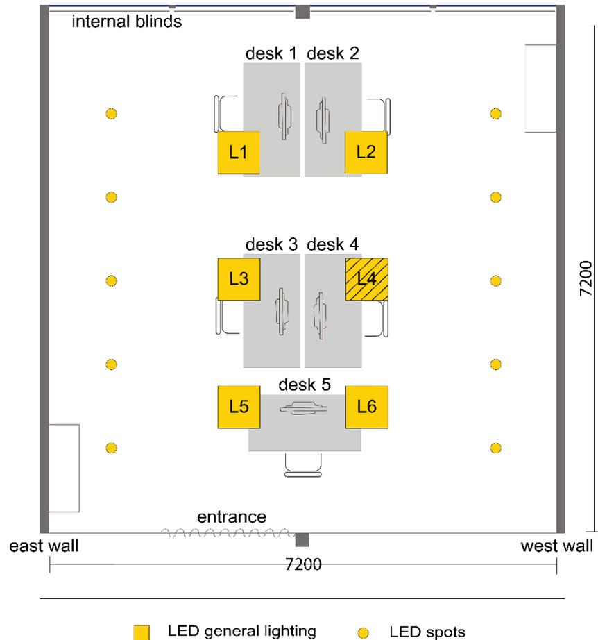
Figure 1. Floorplan of the mock-up office. To simulate occupancy triggered dimming, luminaire L4 was dimmed up and down using different dimming rates.
