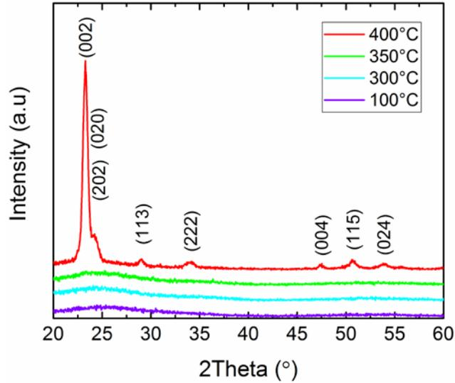
FIG. 7. GI-XRD diffractogram of the  $\text{WO}_3$  films deposited at various temperatures. For the  $\text{WO}_3$  film deposited at 400 °C, the respective peaks are indexed according to monoclinic  $\text{WO}_3$ .
