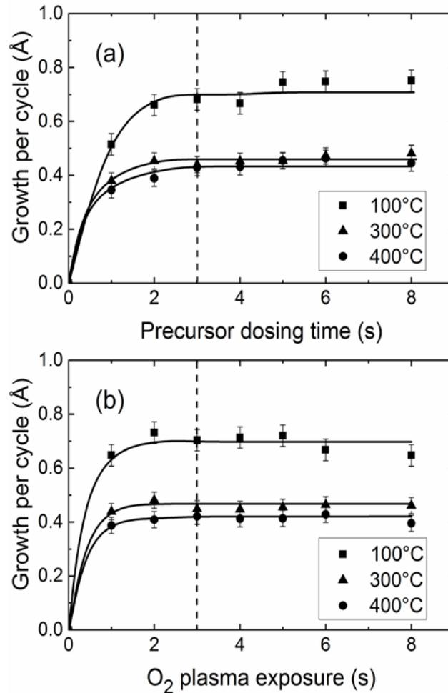
FIG. 2. Saturation curves: GPC as a function of (a) precursor dosing and (b) plasma exposure, for deposition temperatures of 100 °C, 300 °C, and 400 °C. The dotted lines indicate the respective chosen precursor/O<sub>2</sub> plasma saturation times (3s) for the WO<sub>3</sub> ALD process. The solid lines serve as guide to the eye.
