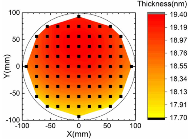
FIG. 4. Thickness uniformity of the  $\text{WO}_3$  film on an 8 inch (200 mm) Si wafer as-determined by room temperature SE mapping. The  $\text{WO}_3$  film was deposited at 200 °C
