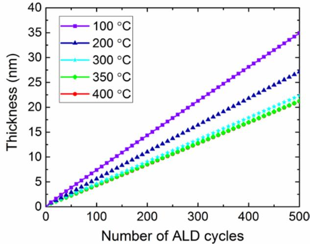
FIG. 1.  $\text{WO}_3$  film thickness in progression of number of ALD cycles for deposition temperatures ranging from 100 °C-400 °C, as-determined by in-situ SE
