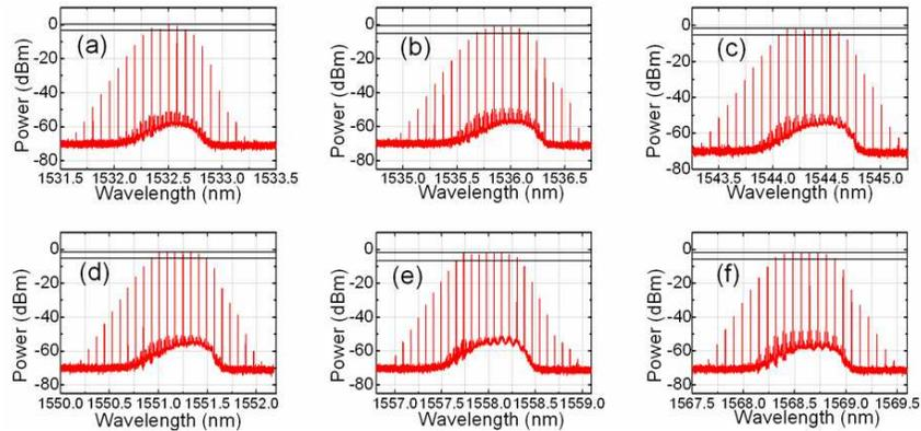
Fig. 3. Optical spectra of external injection seeded, gain-switched optical combs at different operating points (a)-(f) Wavelength tuning range from 1530nm to 1570nm (40nm)
