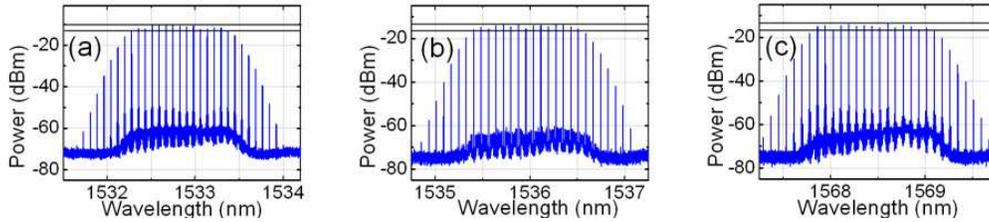
Fig. 4. (a)-(c) Optical combs consisting of 14-16 tones which are expanded via phase modulation.
