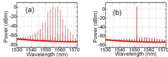
Fig. 2. Optical spectra (a) free running FP-LD @ 40mA bias and (b) externally injected FP-LD.
