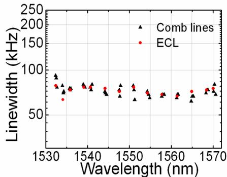
Fig. 5. Optical linewidth of the selected comb lines (black triangle) and the external cavity laser (red circles) at the operating points over the 40nm wavelength range.
