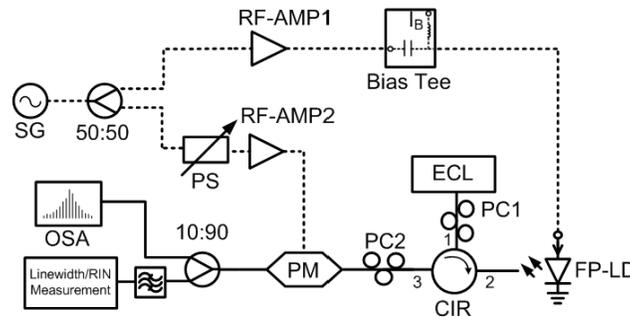
Fig. 1. Experimental setup for the tunable comb generation scheme using an externally injected, gain-switched FP-LD for comb generation, and phase modulation for comb expansion.
