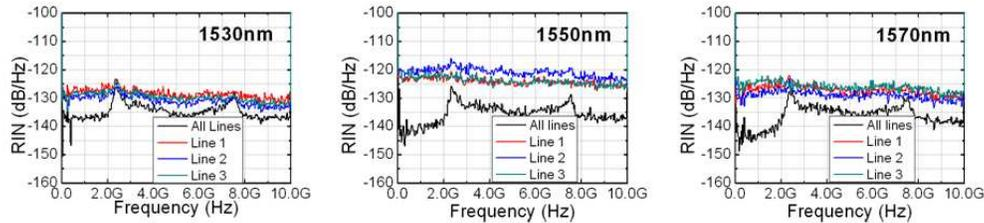
Fig. 6. RIN measurement of the 3 chosen operating modes and of the individually filtered comb lines.
